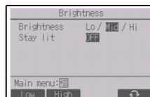
Note: Adjust the brightness to improve viewing in different lighting conditions or installation locations. This setting can not improve viewing from all directions.
